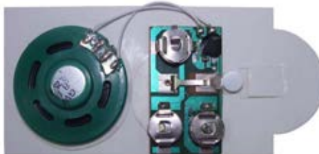
..... Middle: A potentiometer Bottom: A typical sound module taken from a greeting card
